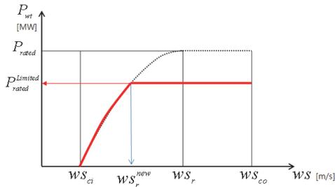
Figure 6: Normal/Restricted Output Characteristic of WT.
