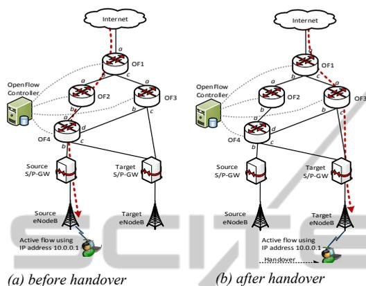
Figure 2: OpenFlow approach to support DMM in a virtualized LTE system.
