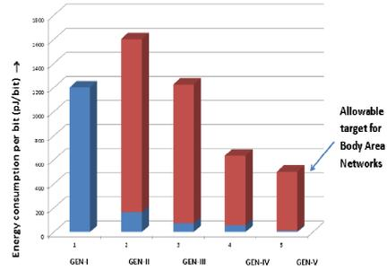
Figure 2: Proposed evolution of next-generation wireless communications IC energy consumption with respect to the allowable targets for BANs, with 0.2 dBm transmit power; Blue - Energy consumption of BB; Red - RF.
