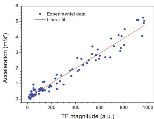
Figure 10: variation of acceleration amplitude obtained from cyclograms versus DFT signal magnitude.
