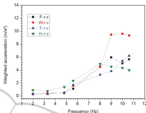
Figure 11: weighted acceleration versus vibration frequency with test bench rocking vibration (r.v) configuration. F: wheelchair footrest; W: wheelchair frame; T: vibrating table; H: user head.
