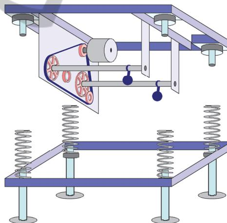
Figure 2: Schematic of the vibrating table.
