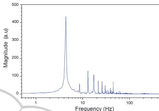
Figure 6: DFT response in semi-log plot of the raw acceleration signal presented in Fig. 4.
