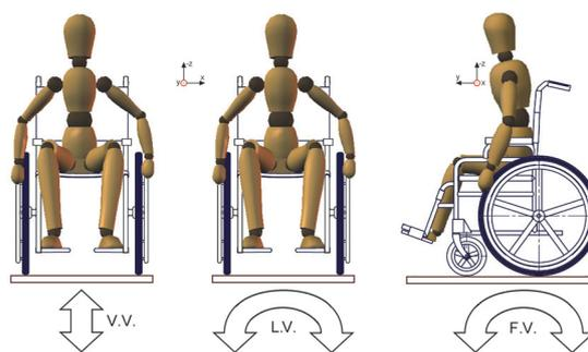
Figure 1: Basic vibrations that can be induced on a manual wheelchair: vertical vibration V.V, lateral vibration L.V and fore-and-aft vibration F.V.
