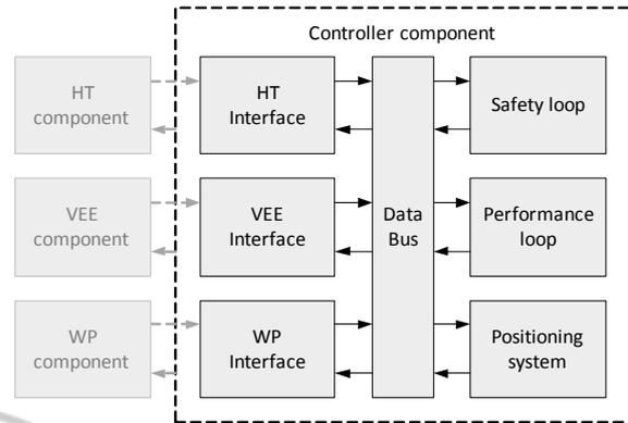
Figure 5: Modules of the Controller component. HT: Home Trainer, VEE: Virtual Exercise Environment, WP: Web Portal.
