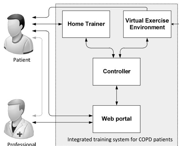
Figure 1: High level architecture of the Integrated Training System.
