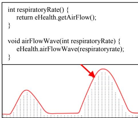
Figure 3: Functions to retrieve respiratory rate and airflow wave.
