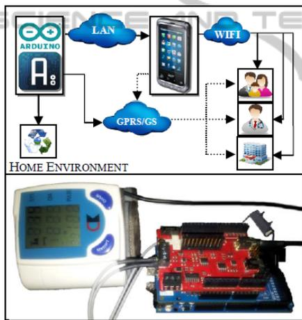
Figure 1: a) Arduino based monitoring system Architecture tracks the user vital signs and sends this information to their mobile. Also, it tracks environment condition and, if is necessary, changes them according to the health status of the user. b) E-Health Monitoring System based on Arduino.
