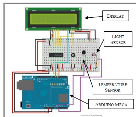
Figure 5: Environment Monitoring System.
