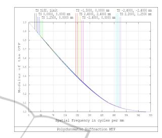
Figure 3: Simulated MTF over 5×5mm FOV.
