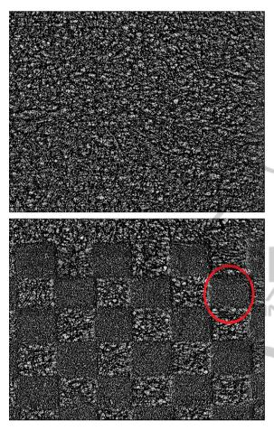
Figure 6: Surface for a blank paper (top) and the same paper with printed stimuli (bottom): for better visualisation, the corresponding SI region to the marked part of the surface (See Figure 5) is circled in red.
