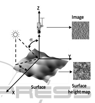
Figure 1: Set-up for capturing images in PS algorithm.
