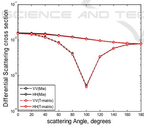
Figure 1: Comparison of Mie-theory and T-Matrix method for differential scattering cross sections of non-absorbing spherical and offset spherical particles at 220 GHz.
