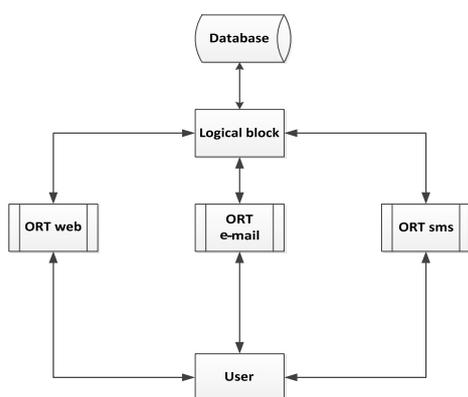
Figure 3: The flow of information between the modules of the system.
