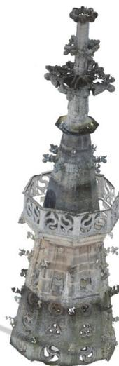
Figure 5: The six point clouds captured from the scaffold registered into a common coordinate system.
