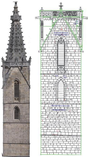
Figure 7: Left: Orthophoto of the tower's south façade, derived from UAV imagery. Right: The corresponding CAD drawing.
