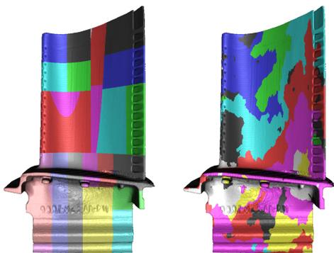
Figure 2: Partitioning of a 883K vertices turbine blade model for rendering with WebGL. Left: Kd-tree-based approach, 32 patches. Right: Vertex cache optimization approach, using the minimum of 14 patches.
