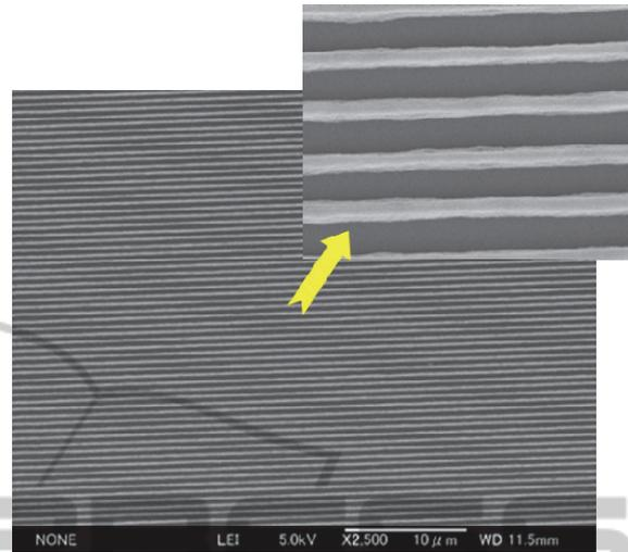
Figure 3: SEM image of the grating pattern fabricated by laser interference lithography.
