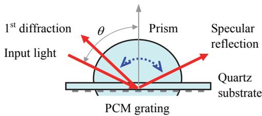
Figure 1: Schematic of the proposed optical switch by PCM grating. Light is coupled in and out by the top semi-cylindrical prism. The incidence angle of input light is indicated by  $\theta$ .
