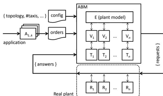
Figure 2: Architecture of an ABM controller.
