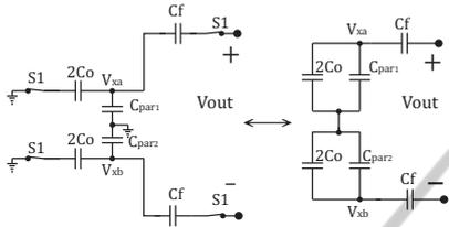
Figure 5: Equivalent schematic for determining the feedback factor (13).
