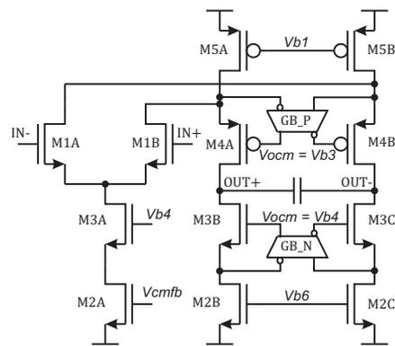
Figure 10: The gain boosted folded cascode amplifier.
