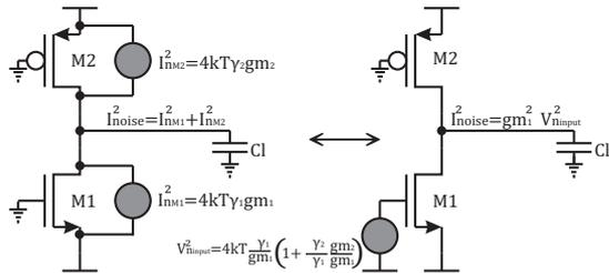
Figure 8: Input referred system noise current.
