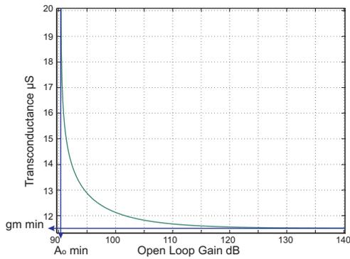
Figure 11: Plot of  $g_m$  versus  $A_0$  from (35) for  $f_{sc} = 4\text{kHz}$  showing asymptotic behavior at minimum  $g_m$  and minimum  $A_0$ .
