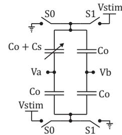
Figure 1: The capacitive pressure sensor as part of a capacitive bridge.
