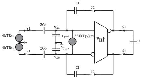
Figure 6: Schematic of the SC amplifier during phase S1.
