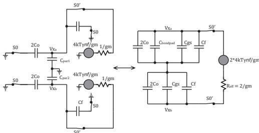
Figure 3: Schematic of the SC amplifier during phase  $S_0$ .
