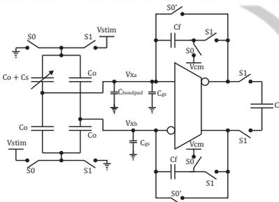
Figure 2: Schematic of the capacitive bridge and the SC amplifier with associated parasitic capacitances.
