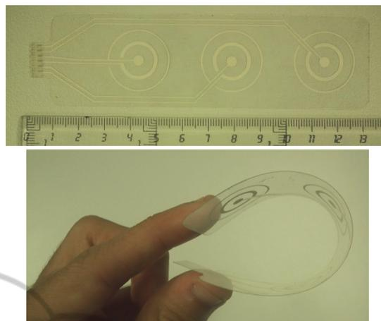
Figure 3: Implemented flexible array of three TCB concentric ring electrodes.
