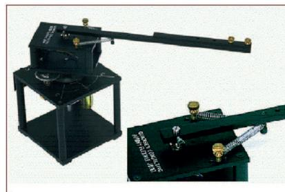
Figure 1: Physical model of flexible joint robot manipulator.
