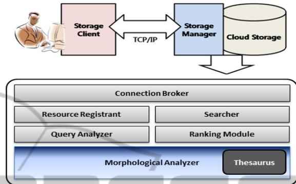
Figure 1: Model Repository Architecture in OpenSIM.
