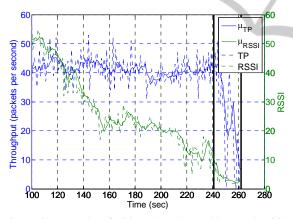
Figure 3: Example of video throughput (blue) and RSSI data (green) received at the OCU from a *PackBot* using the MDCR system. Solid line is the average ( $\mu$ ) of past five samples of underlying (dotted) data. Left and right black lines represent t<sub>F</sub> and t<sub>L</sub>, respectively.
