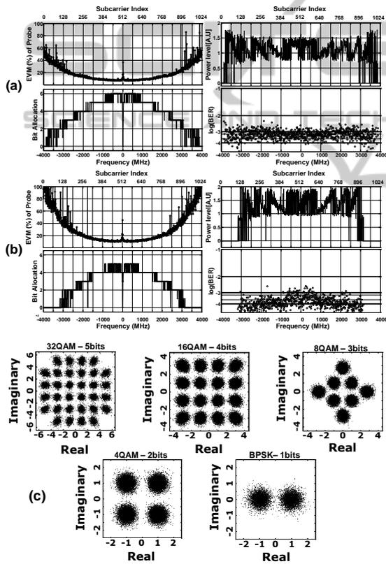
Figure 3: Probe EVM, adaptive bit and power loading profile, BER each data subcarrier and constellation of maximum bit loading subcarriers: (a) optical back-to-back (data rate: 29.68 Gb/s, average BER:  $9.79 \times 10^{-4}$ ), (b) 20-km bi-directional (data rate: 21.59 Gb/s, average BER:  $4.57 \times 10^{-4}$ ); (c) recovered signal constellation for the 20-km bi-directional case.
