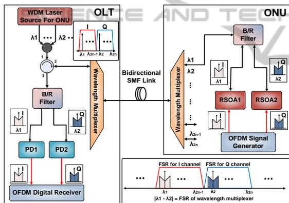
Figure 1: Proposed optical OFDM/WDM PON using separated I/Q baseband delivery for colorless ONU.
