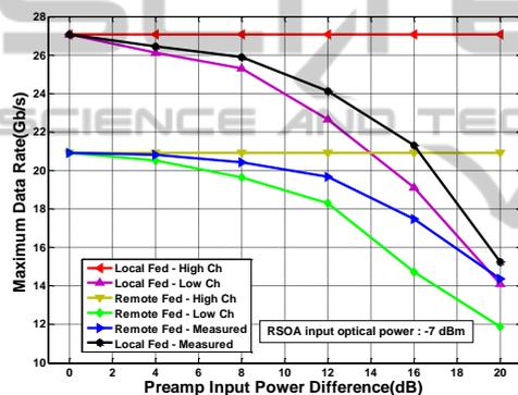
Figure 5: Maximum achievable data rate with various input optical power deviation of the preamplifier power between I/Q channels.
