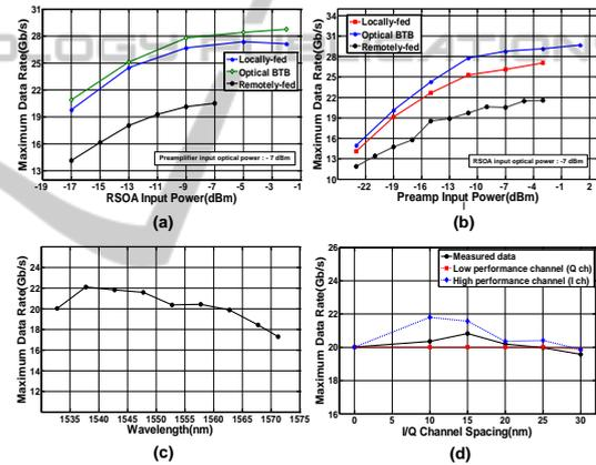
Figure 4: Maximum achievable throughput as a function of: (a) input optical power of the RSOA, (b) input optical power of preamplifier, (c) various wavelength, (d) I/Q channel wavelength spacing.
