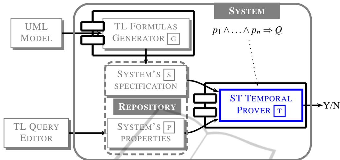
Figure 4: Deduction-based verification system.
