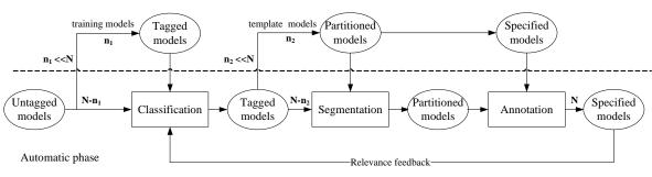
Figure 2: The framework of our method for specifying semantics of 3D models.
