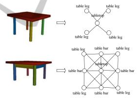
Figure 4: Segmented models are represented by AAG.
