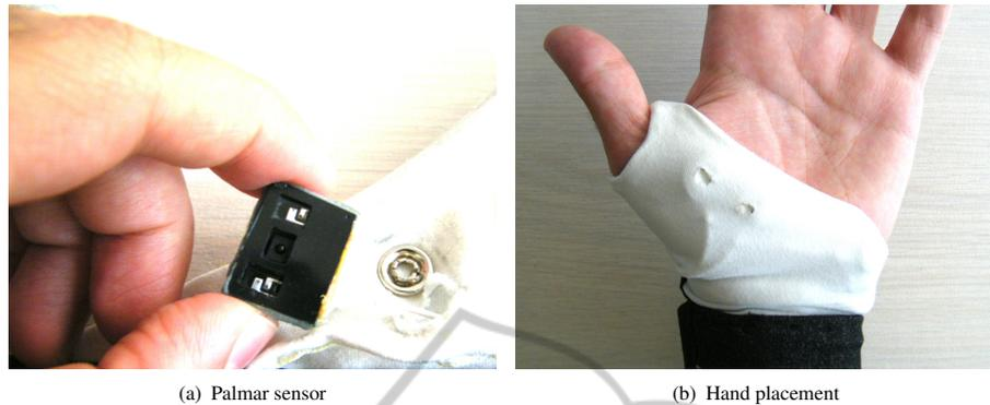
**Fig. 2.** Blood Volume Pulse (BVP) sensor and placement at the hand palm.
