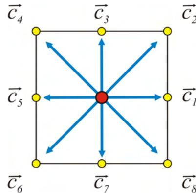
Figure 1: The D2Q9 LBM node, with 8 non-zero velocities.
