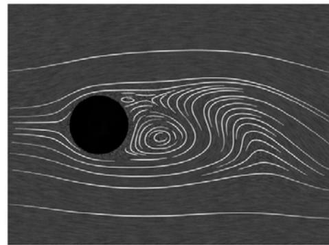
Figure 8: An illustrative flow past a cylinder with Reynolds number 100. (Source: (Schroeder et al., 2010))
