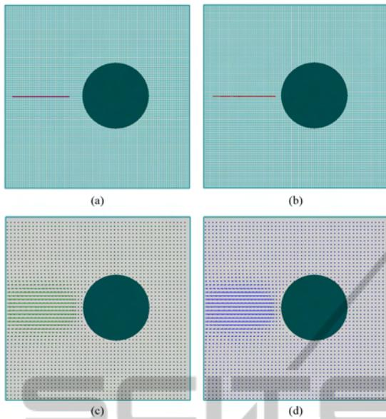
Figure 6: Example 2: flow of a gas with a solid object. (a) The sketching. (b) The tangent field. (c) The initial velocity field given by the GVF. (d) The LBM initialization through the field in (c).
