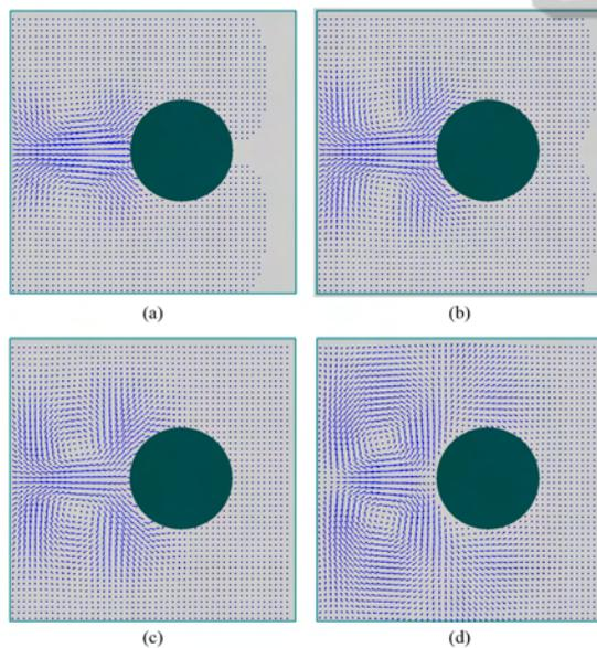
Figure 7: Example 2: the evolution of the fluid simulation. The sequence (a)-(d) shows four instants of the LBM simulation, which was initialized using Figure 6(d) as initial velocity condition.
