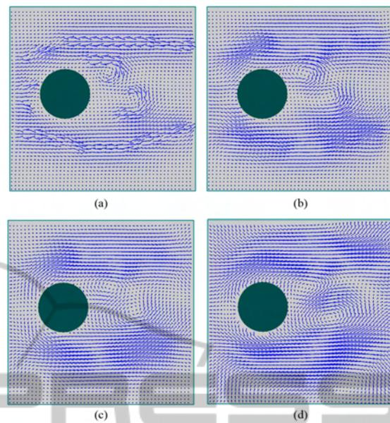
Figure 5: Example 1: the evolution of the fluid simulation. The sequence (a)-(d) shows four instants of the LBM simulation, which was initialized using Figure 4(d) as initial velocity condition.
