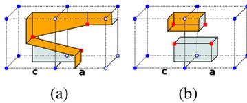
Figure 2: Possible patches for two 6 solid vertices cells connected by an ambiguous face. (a) solid component, (b) empty component. Dual vertices are noted as red squares.
