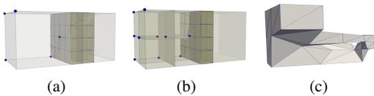
Figure 4: Two neighbours cells are illustrated, blue spheres are cells corners inside  $F(x)$ . Collapsed cell (left) is in clear, deeper cells are in dark. (a) Our algorithm detects a complex face and subdivides the left cell (b), (c) The tunnel between cells is captured and a manifold surface is generated.
