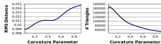
Figure 8: RMS distance and number of triangles for Wales Dragon data set with respect to the curvature parameter  $\delta$ .
