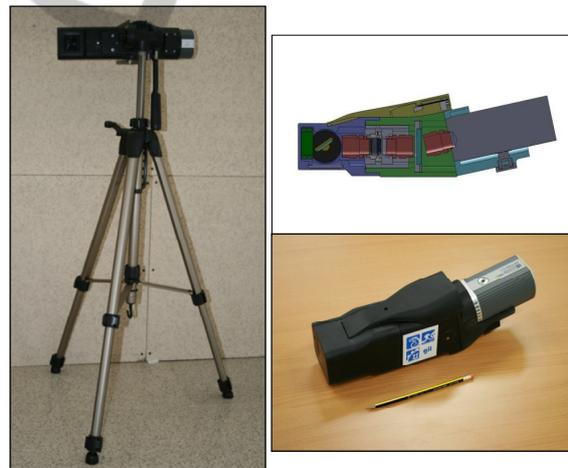
Figure 1: Hyperspectrometer designed and built for this project.
