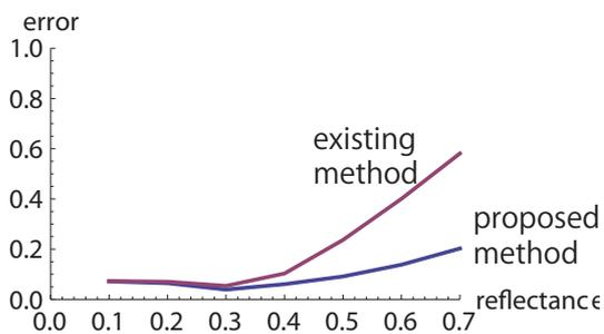
Figure 11: The accuracy of estimated light source distributions. If the reflectance of the reference object is large, the accuracy of the existing method (Sato et al., 2003) degrades drastically, while that of the proposed method does not.
