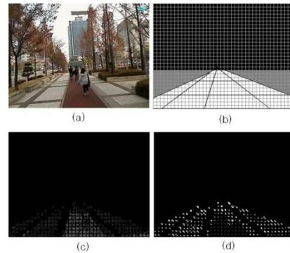
Figure 9: Result of texture feature extraction within triangular model, (a) original image, (b) triangular model based on 8x8 window, (c) rotation invariant LBP, (d) GLCM.
