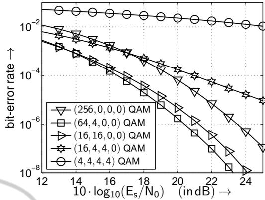
Figure 7: BER when using the transmission modes introduced in Tab. 1 and transmitting 8 bit/s/Hz over correlated frequency non-selective channels (linear distribution of both the transmit and receive antennas with  $\Delta_t = 10$  and  $\Delta_r = 4$ ).
