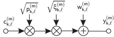
Figure 1: Resulting  $k$ th user-specific system model per MIMO layer  $\ell$  (with  $\ell = 1, 2, \dots, n_{\mathbf{R}_k}$ ) and per transmitted symbol block  $m$
