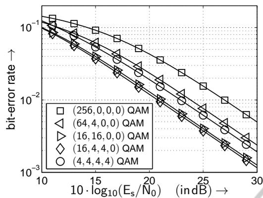
Figure 9: SVD-based user-specific BERs when using the transmission modes introduced in Table 1 and transmitting 8 bit/s/Hz over uncorrelated frequency non-selective channels.
