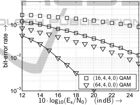
Figure 8: BER with linear antenna distribution (solid line) and with non-linear antenna distribution (dotted line) when using the transmission modes introduced in Tab. 1 and transmitting 8 bit/s/Hz over correlated frequency non-selective channels ( $\Delta_t = 10$  and  $\Delta_r = 0,1$ ).
