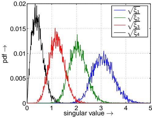
Figure 5: PDF (probability density function) of the layer-specific amplitudes  $\sqrt{\xi_\ell}$  for uncorrelated frequency non-selective MIMO channels.
