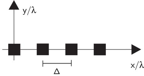
Figure 2: Linear antennas distribution.
