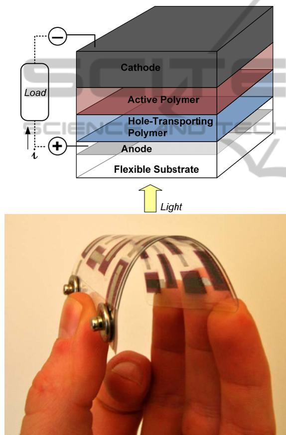
Figure 1: Structure of a generic polymer solar cell and photograph of a working polymer solar panel. The panel consists of 12 cells connected in series and can generate 5V in outside light.
