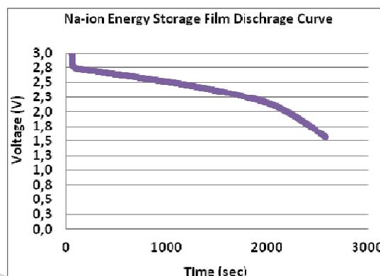
Figure 6: Discharge profile for a single PES cell with a constant current load of 100uA charged with 5V.
