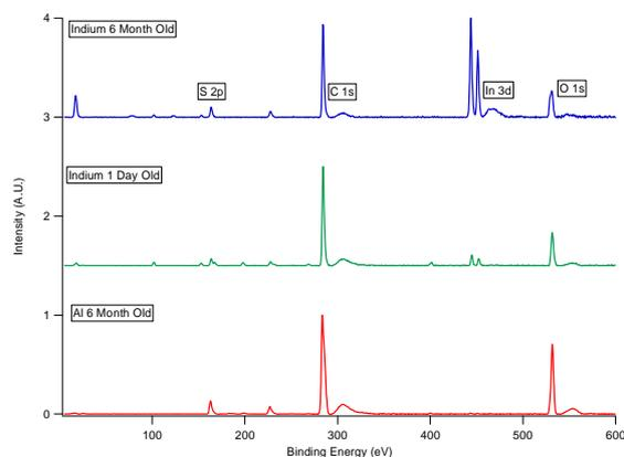
Figure 2: Broad-spectrum scans of Aluminium Cathode vs. Indium Cathode based PSCs.
