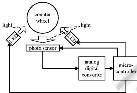
Figure 1: Structure of the measurement system.
