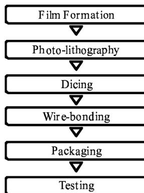
Figure 1: Six major stages of SAW manufacturing processes.
