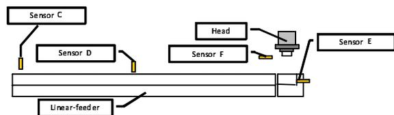
Figure 3: Locations of sensors along the linear-feeder.
