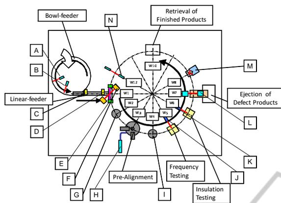
Figure 2: Structure of a testing machine.
