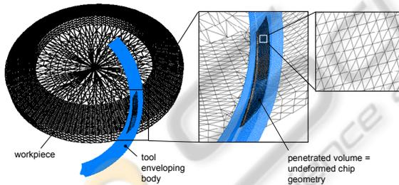
Figure 6: 3D penetration calculation of triangulated surfaces.
