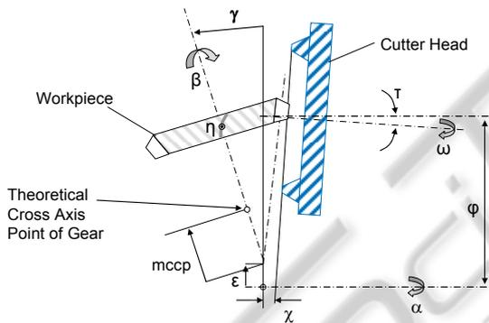
Figure 2: Scheme and axis movements of a bevel gear cutting machine.
