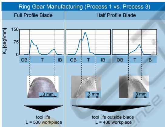
Figure 14: Comparison of different tool concepts
