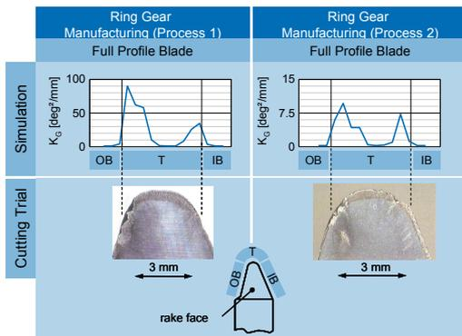
Figure 11: Tool wear analysis of full profile blades.
