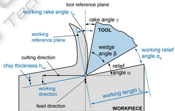
Figure 7: Calculable characteristic values.
