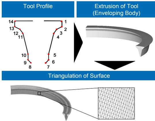
Figure 5: Modelling and triangulation of tool.
