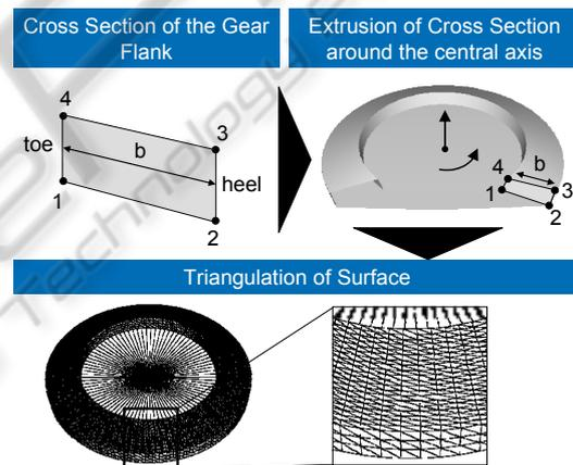
Figure 4: Modelling and triangulation of workpiece.
