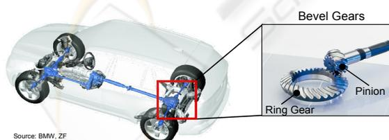
Figure 1: Exemplary automotive application of bevel gears.
