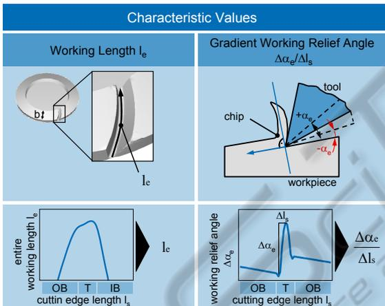
Figure 10: Working length and gradient of relief angle.
