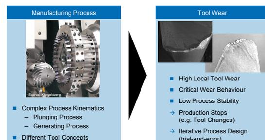
Figure 2: Challenges in bevel gear cutting.
