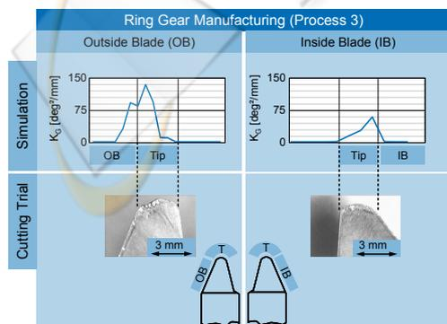
Figure 12: Tool wear analysis of half profile blades.
