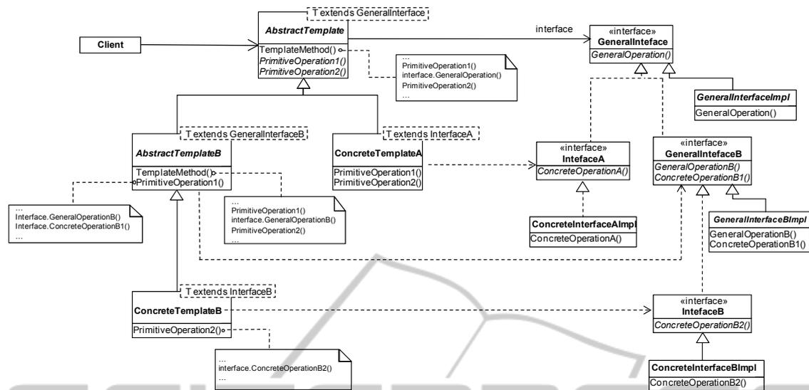
Figure 8: Decoupling the *Interface* abstraction from its implementation.
