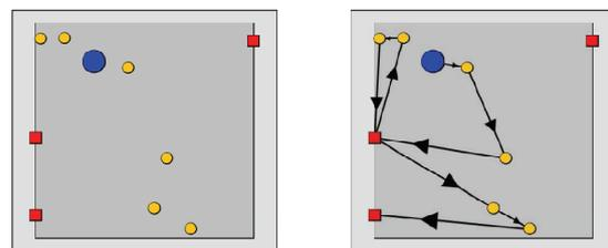
Figure 1: Example of 6+3 robot planning task. The robot (the big circle) collects waste (six small circles) and uses collectors (three squares) to empty the bin when it is full.
