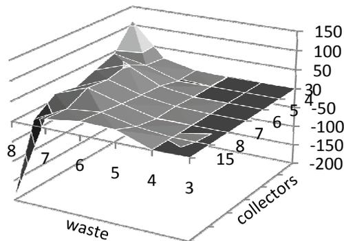
Figure 6: Time difference (seconds) between the CP models. Positive values means that the model based on finite state automata is faster.
