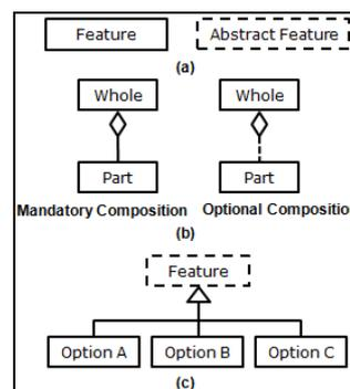
Figure 1: FAM Notation (a) Feature types, (b) Composition relation, (c) Generalization/ Specification relation.
