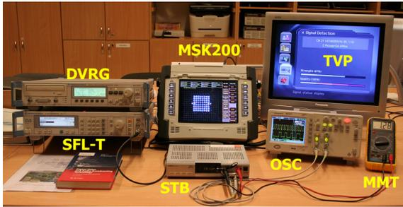
Figure 3: Laboratory workplace for the DVB-T measurements and transmission link.
