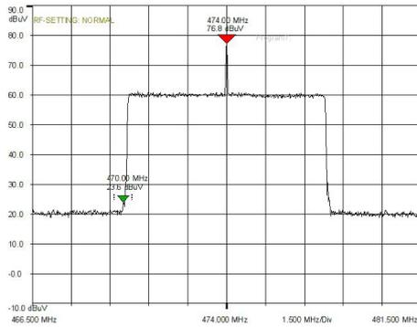
Figure 8: DVB-T spectrum without suppressed carrier, C21 (470 – 478) MHz, 8k mode, CS = 50% (CS error visible at central carrier, 474 MHz).
