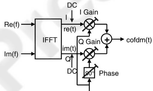
Figure 1: DVB-T modulator with I/Q errors and imperfections (Fisher, 2008).
