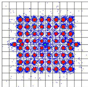
Figure 5: I/Q constellation of the DVB-T, 64-QAM, 8k mode and in case of CS = 50% presence (CS error visible in the centre of the diagram).
