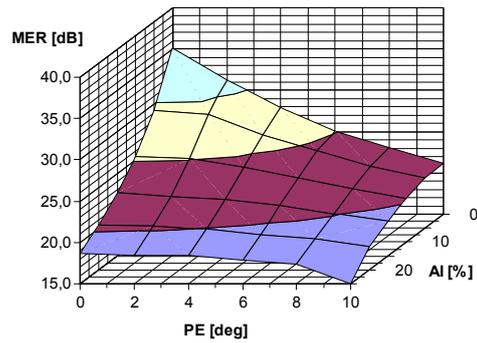
Figure 6: DVB-T modulator imperfections and I/Q errors measurements (simultaneous *AI* and *PE*).
