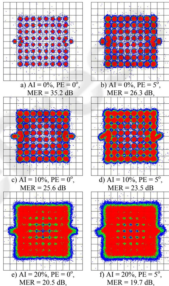
Figure 7: I/Q constellation of the DVB-T with 64-QAM, 8k mode and in case of *AI* and *PE* presence (DVB-T channel correction and all pilots ON).
