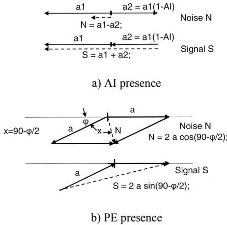
Figure 2: Determining SNR by vector diagrams in case of I/Q errors (Fisher, 2008).
