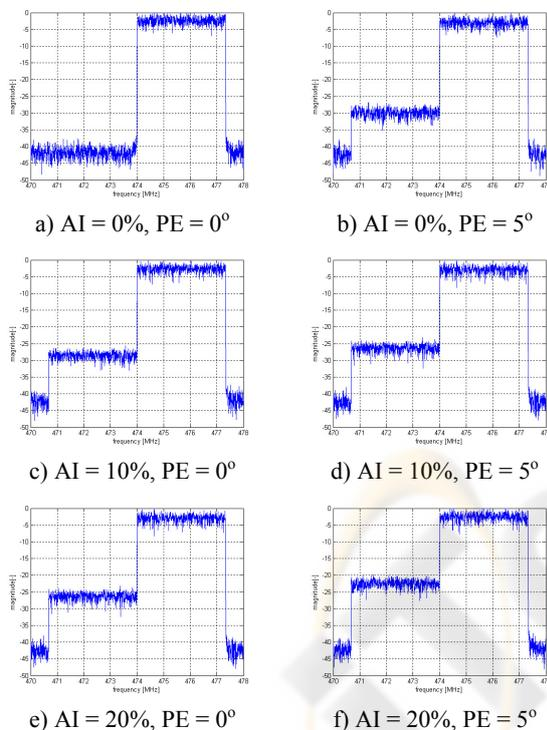
Figure 9: Simulated spectrum of the DVB-T with 64-QAM, 8k mode and in case of AI and PE presence (lower band carriers 0 - 3407 were set to zero to illustrate the crosstalk).
