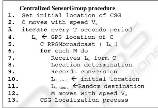
Figure 4: CSG operation procedure.
