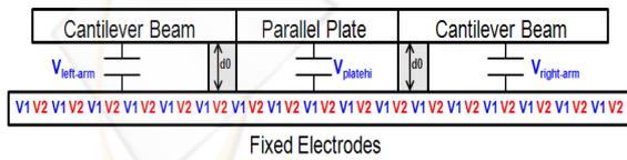
Figure 6: Illustration of different voltage across the beams and the plate capacitor due to disconnection from the parallel plate body.
