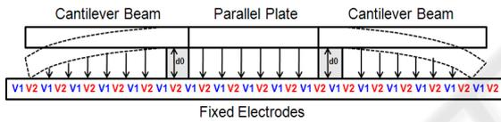
Figure 5: Deformation in cantilever and parallel plate due to applied voltage.
