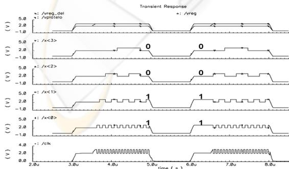
Figure 8: Simulation result of 4-bit counter.
