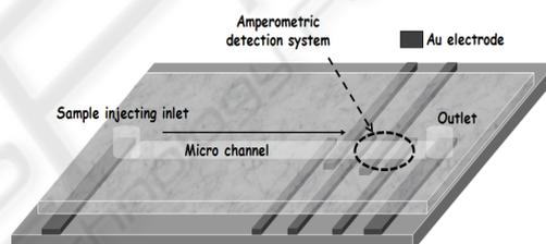
Figure 2: Schematic of PDMS/Glass device.
