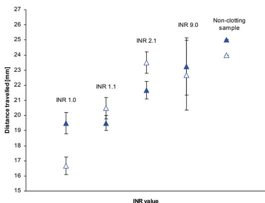
Figure 5: Distances travelled by samples with INR of 1.0 (normal clotting control), 1.1, 2.1, 9.0 and non-clotting. Chips containing 4-fold concentrated PT:RVV at a 1:1 ratio (empty symbols) and 4-fold concentrated PT : RVV : water at 1:1:2 ratio (filled symbols) were used for testing (n=3).
