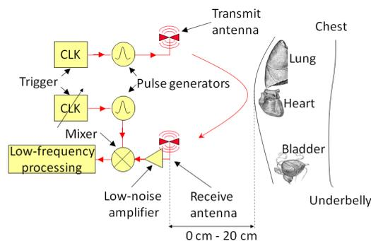
Figure 1: Concept of the on-body water detection system.
