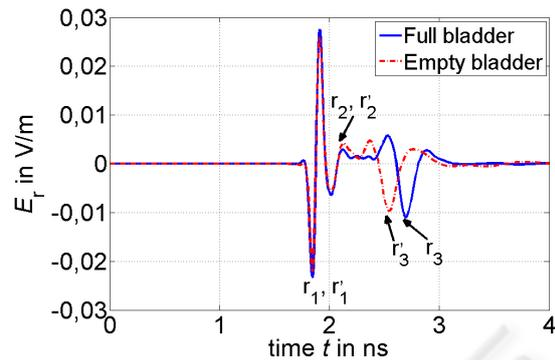
Figure 4: Received electric field  $E_r$  of the UWB pulses by the probe: full (solid) vs. empty (dotted) bladder. (full case:  $r_1$ ,  $r_2$  and  $r_3$ ; empty case:  $r'_1$ ,  $r'_2$  and  $r'_3$ ).
