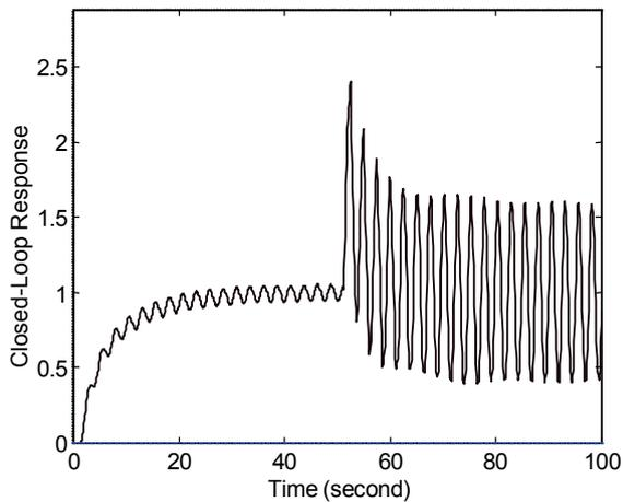
Figure 11: Closed-loop servo-response and regulatory control response of the system  $G(s)=(5s+1)\exp(-1.2s)/(2s+1)(s+1)$ , in the case of the PD-1F controller with parameters  $K_I=0.2208$ ,  $K_P=0.6624$ ,  $K_d=0.3759$ .
