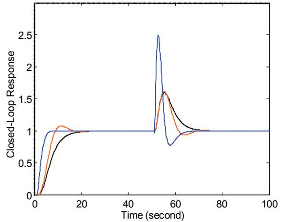
Figure 13: Closed-loop servo-response and regulatory control responses of the system  $G(s)=(5s+1)\exp(-1.2s)/(2s+1)(s+1)$ . Black line: PD-1F controller with filtered output tuned according to relations (17)-(19); Orange line: PD-1F controller with filtered output tuned according to relations (26)-(28); Blue line: Series form PID controller with filtered derivative tuned according to the method in Chien *et al* (2003).
