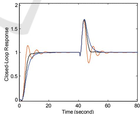
Figure 5: Servo-responses and regulatory control responses for the system  $G_p(s)=(-0.5s+1)\exp(-0.8s)/(s+1)$ , in case of nominal process parameters, for  $\alpha=0.6$  and for three values of  $\beta$ . Orange line:  $\beta=2.05$ ; Black line:  $\beta=2.15$ ; Blue line:  $\beta=2.25$ .
