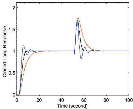
Figure 6: Servo-responses and regulatory control responses for the system  $G_p(s)=(-0.5s+1)\exp(-0.8s)/(s+1)$ , in case of nominal process parameters, for  $\beta=2$  and for three values of  $\alpha$ . Orange line:  $\alpha=0.45$ ; Black line:  $\alpha=0.5$ ; Blue line:  $\alpha=0.55$ .
