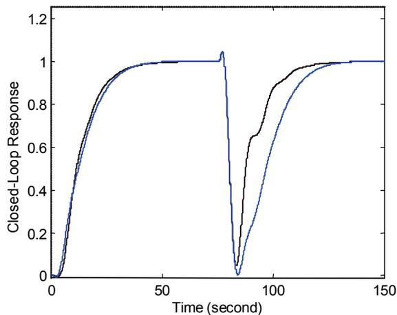
Figure 9: Servo-responses and regulatory control responses for the system  $G(s)=(-s+1)\exp(-0.939s) / [(2.07s+1)(5s-1)]$ . Black line: Proposed method; Blue line: Method in Lee *et al* (2000).
