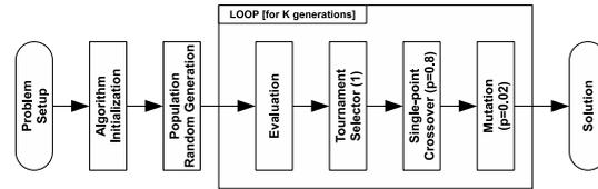
Figure 1: Algorithm structure.
