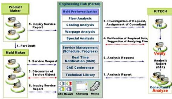
Figure 1: Process of CAE analysis in engineering hub.
