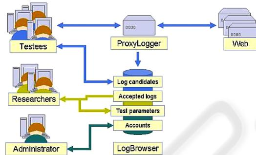
Fig. 1. PLogger architecture.
