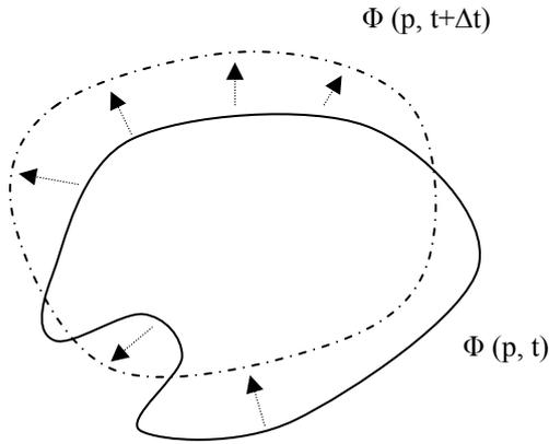
Figure 1: Evolution of a closed curve  $C$  represented by a function  $\Phi$  between time intervals  $t$  and  $t+\Delta t$ .
