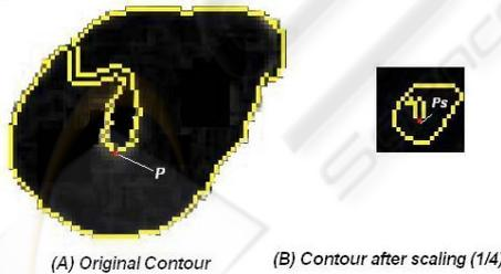
Figure 6: Original Contour (A) and the generated Contour (B) after scaling, the point  $P_s$  (red) after scaling corresponds to the point P (red) of the original contour, so the point  $P_s$  corresponds to more than one point P (approx. 4 points for a scale value of 4) of the original contour.
