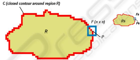
Figure 4: The region  $R_s$  is derived from region R after scale factor applying in the image.
