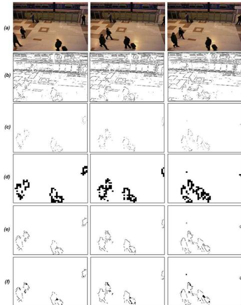
Figure 5: (a) 520<sup>th</sup>, 530<sup>th</sup>, 540<sup>th</sup> frames of PETS2006 dataset; (b) edge map detected by the proposed method; (c) moving edge extraction result; (d) region marking based on moving edges; (e) AND operation between marked regions and edges using Canny operator; (f) after morphological closing.
