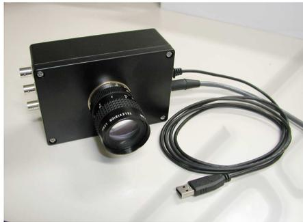
Figure 4: Lock-in camera using 3PCIS. This enables parallel correlation detection with two arbitrary analog orthogonal reference signals supplied in the three-phase form. The three correlation outputs are A/D-converted and transferred to a PC via the USB.
