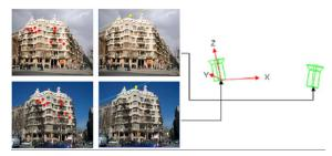
(a) Epipolar geometry and matching points with automatic feature detection and matching (b) Recovered 3D camera position with SIFT and RANSAC
