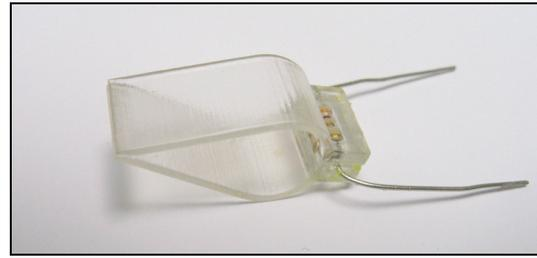
Figure 3: Epoxy resin pincer with built-in heating resistor for activation.
