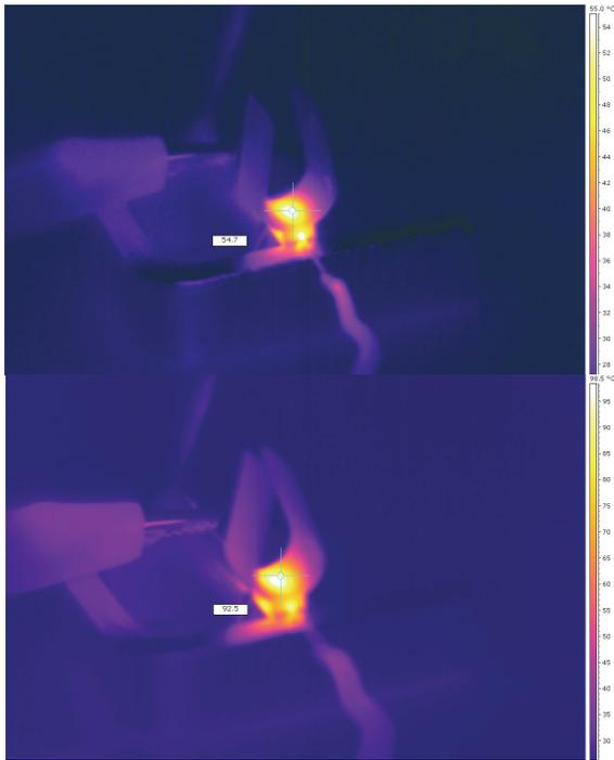
Figure 5: Infrared thermograph of the pincer during the heating process, below (54.7°C) and above (92.5°C) activation temperature.
